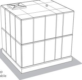
A 9,200 litre TIF tank shown mounted on a concrete slab base. This is one of the recommended methods of tank support structure suitable for TIF tanks.
